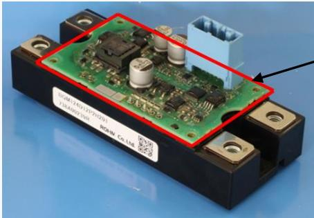
Gate driver PCB: 84.7mmx49.6mm/6 layers
