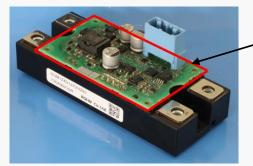
Gate driver PCB: 84.7mmx49.6mm/6 layers
